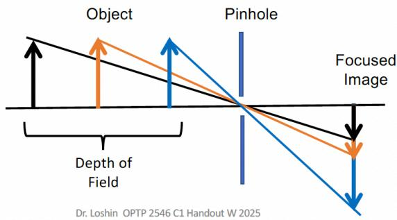
**Depth of Focus:** the range over which the image screen can be moved and maintain a clear image
