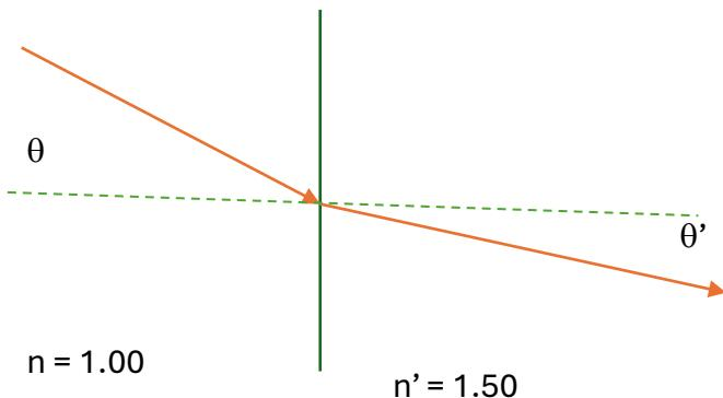
Note that the ray of light is refracted toward the normal when traveling from a rarer medium (lower index) to a denser medium (higher index).
